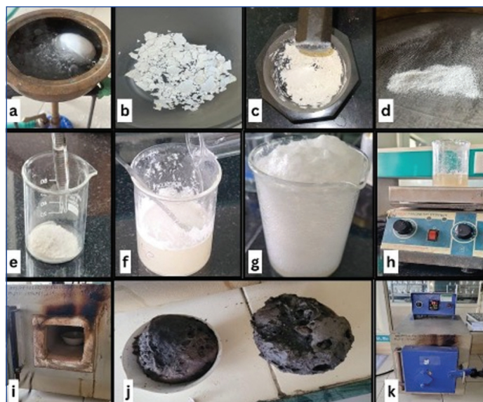
[Table/Fig-1]: Sequential preparation of Eggshell Powder (ESP): a) Boiling of eggshells; b) cleaned and crushed eggshells; c) grinding into fine particles; d) sieving of the powder after calcination in a muffle furnace; e) dissolution in nitric acid; f) addition of diammonium hydrogen phosphate; g) formation of a white precipitate; h) development of a transparent gel; i) heating of the gel at 250°C; j) formation of a black precursor; and k) sintering at 900°C for 2 hours to obtain the final white Eggshell Powder (ESP).
